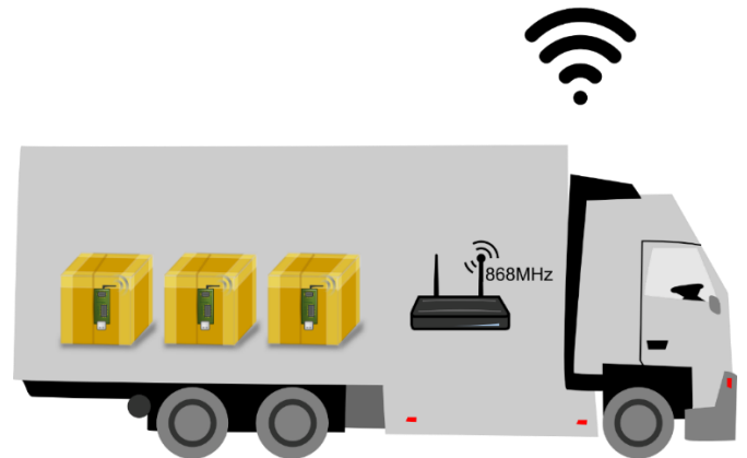
Figure 2 One gateway provides LoRaWAN for all shipments inside the truck [4]
